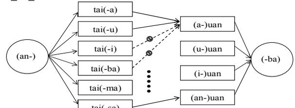
Fig. 3 Possible links between the synthesis units for synthesizing /tai uan/
