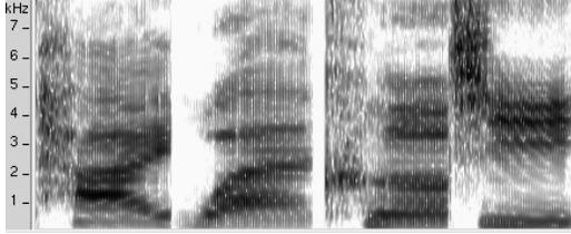
Fig. 1 Spectrogram for a synthetic speech of "台灣科技".
